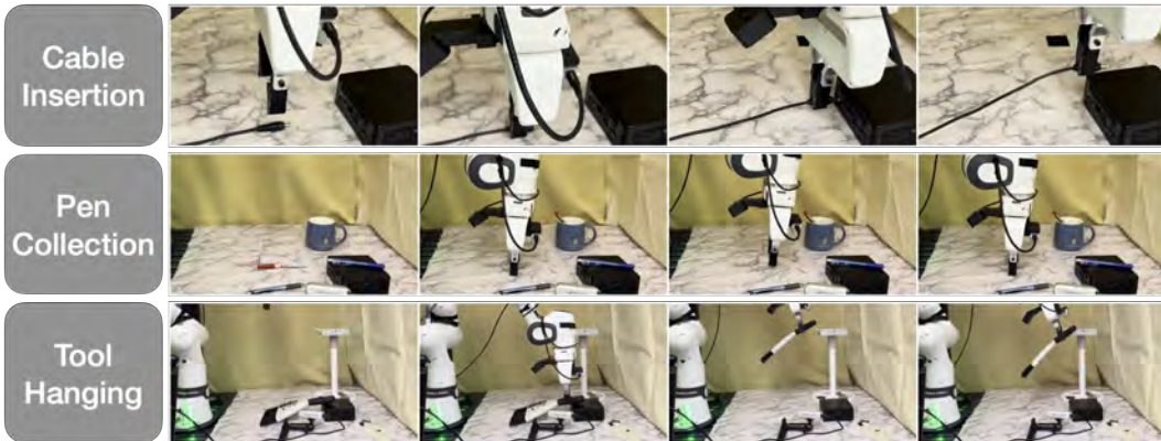
Figure 8: Failure rollouts of PATCH POLICY for Cable Insertion, Pen Collection, and Tool Hanging.
